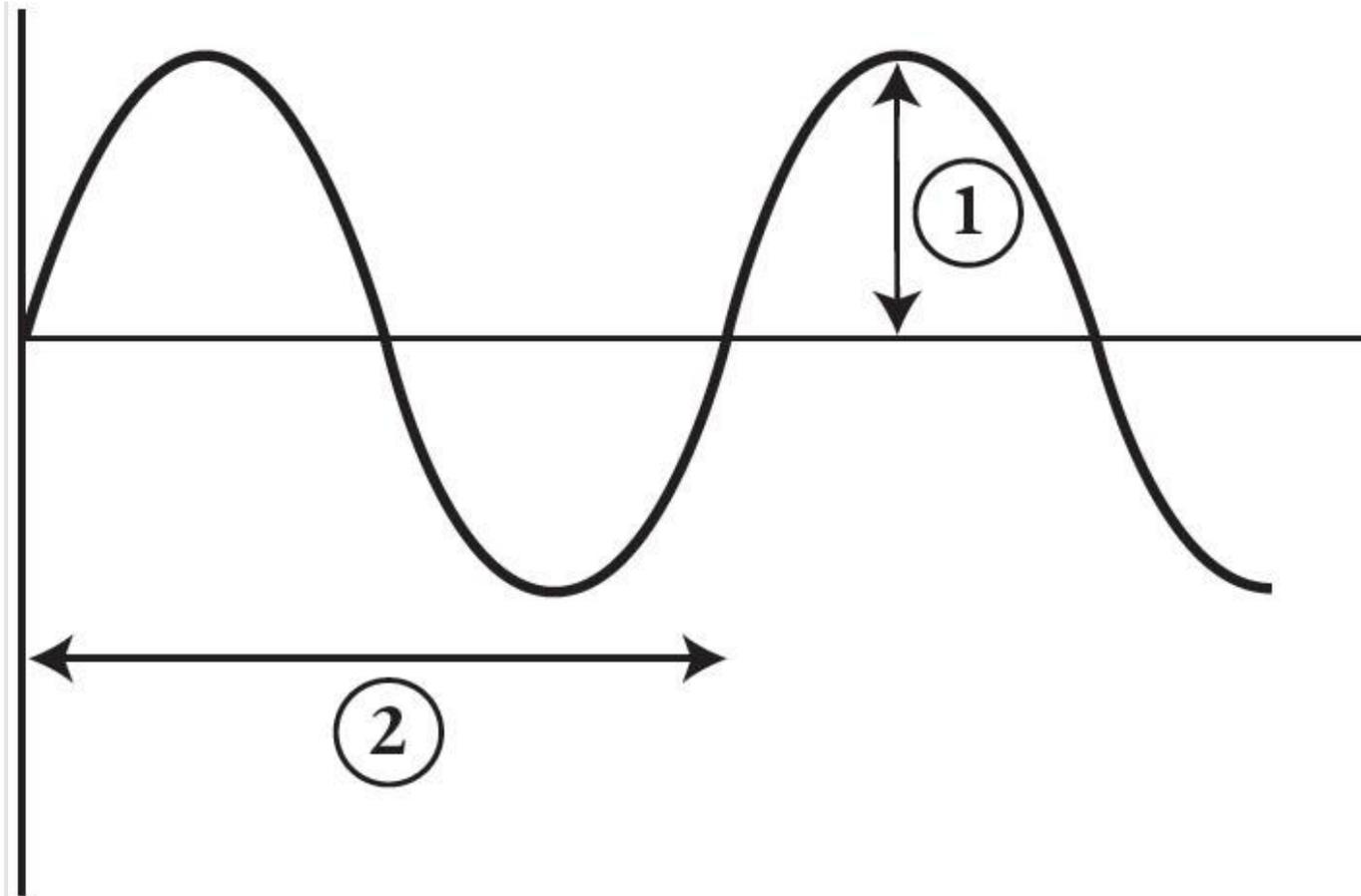
The amplitude (1) is simply the maximum amount of energy the wave has, and the frequency (2) is the number of times that the wave repeats each second. The frequency is usually measured in units referred to as hertz, or 'Hz' for short. To understand the difference between amplitude and frequency, it's helpful to sing a little song. Please sing 'Laaaa' in a deep voice. You have just produced a low-frequency note that would look something like the top line in the following diagram.
