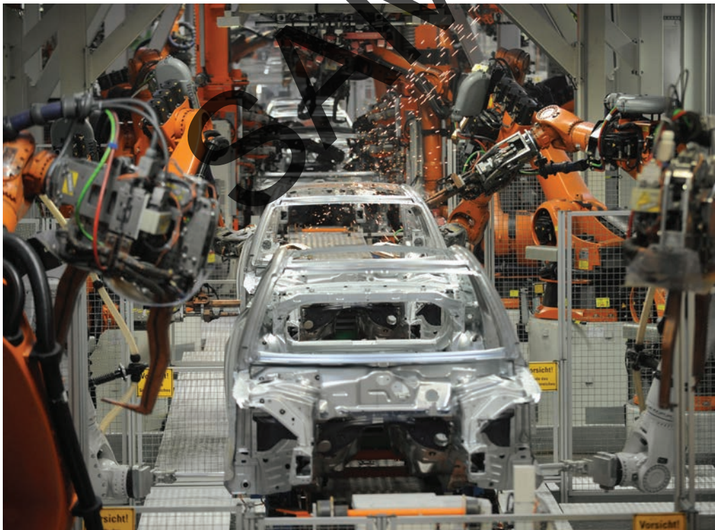
The use of computer-controlled robots has increased productivity in car manufacturing
