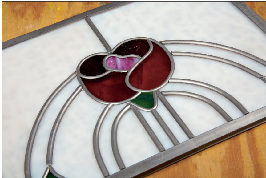
Figure 1-3: Several unsoldered lead inter- sections, also called joints.
