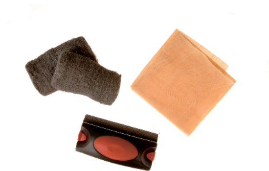
Figure 1-4: Steel wool pads, sanding block with sandpaper, and a tack cloth.
